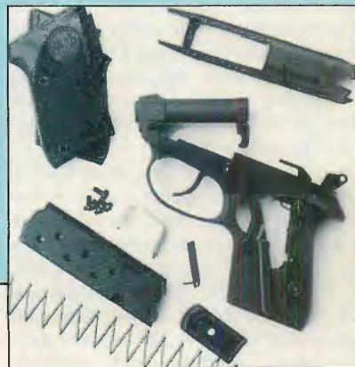
Beretta Model 3032 Tomcat, fieldstripped.
